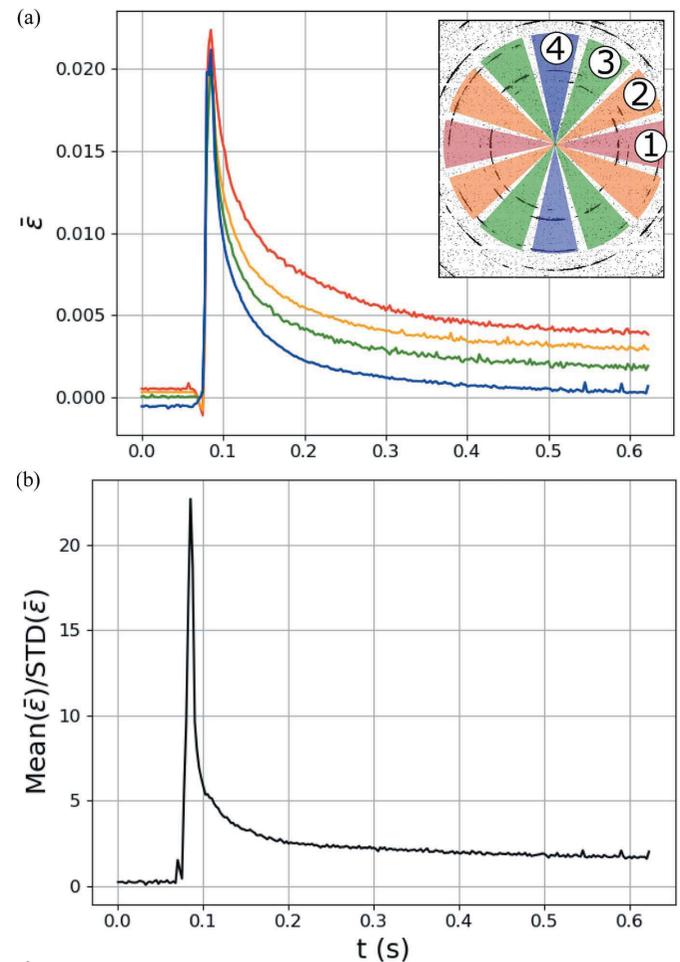
**Figure 11** (a) Evolution of average lattice strains  $\bar{\epsilon}$  measured from four different regions on the detector (shown in inset) through time  $t$ . (b) Evolution of the ratio of the mean and standard deviation (STD) of the lattice strains from the four different regions.
