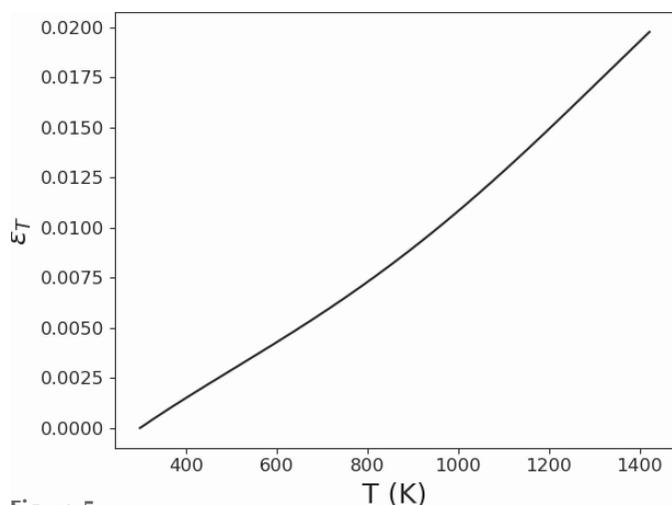
**Figure 5** Measured thermal strain  $\varepsilon_T$  versus temperature  $T$  of IN625 used for the diffraction simulations. Measurements were made using dilatometry on the same material as tested in the synchrotron experiment.
