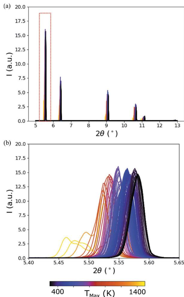
**Figure 7** Simulated (a) diffraction line profiles ( $I$  versus  $2\theta$ ) and (b) 111 diffraction peaks of IN625 colored by the maximum temperature ( $T_{Max}$ ) in the diffraction volume, which was used to generate the pattern.
