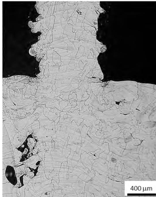
**Fig. 6.17.** Lack of fusion bulk defects, and rough surface of a Ti-5553 laser PBF processed lattice structure component [491].
