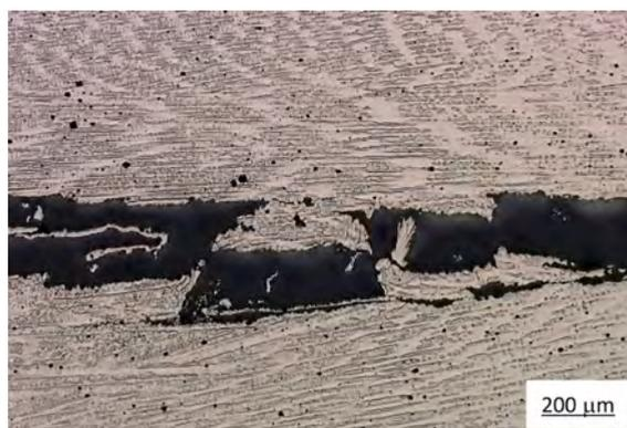
Fig. 7.5. An optical micrograph showing cracking in a DED-GMA 3 wt%Si bronze alloy 3D shape, where the cracks form at the columnar grain boundaries growing parallel to the build direction (etched in nitric acid) [528].
