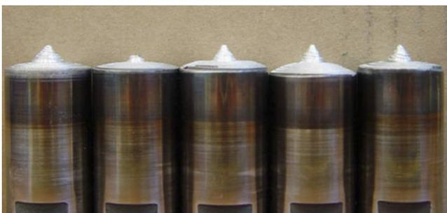
**Fig. 13** The tools used by Neilsen during FSW of AA7075 after use. The tool pin in the second tool from the left sheared off during welding [35]
