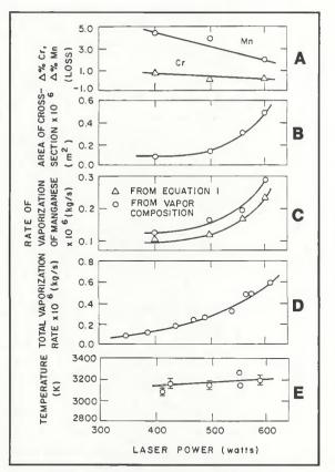
Fig. 2 – Effects of laser power on: A – change in weld composition; B–cross-sectional area; C–rate of vaporization of manganese; D – total vaporization rate; E – weld pool temperature in conduction mode of welding. Steel type: AISI 202; welding speed:  $3 \times 10^{-3}$  m/s; shielding gas flow rate:  $1 \times 10^{-4}$ m<sup>3</sup>/s of He; sample thickness:  $0.7 \times 10^{-3}$  m
