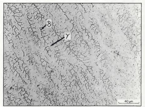
Fig. 12 – Microstructure of laser beam welded AlSI 201 high-manganese stainless steel. Welding speed:  $15 \times 10^{-3}$  m/s; laser power: 4000 W; argon (shielding gas) flow rate:  $5.5 \times 10^{-4}$  m<sup>3</sup>/s
