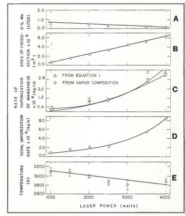
Fig. 3–Effects of laser power on: A–change in weld composition; B– cross-sectional area; C–rate of vaporization of manganese; D–total vaporization rate; E– weld pool temperature in keyhole mode of welding. Steel type: AISI 201; welding speed:  $15.24 \times 10^{-3}$  m/s; shielding gas flow rate:  $5.5 \times 10^{-4}$  m<sup>3</sup>/s of Ar; sample thickness:  $2.5 \times 10^{-3}$  m
