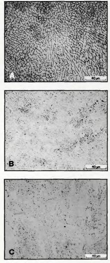
Fig. 9 – Microstructures of laser beam welded AISI 200 high-manganese stainless steel observed at different welding speeds. Laser power: 400 W; Welding speed – A –  $2.2 \times 10^{-3}$  m/s; B –  $13.2 \times 10^{-3}$  m/s; C –  $35 \times 10^{-3}$  m/s
