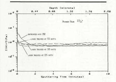
Fig. 6 – Relative counts of H/Fe as a function of sputtering time for samples welded at various laser powers. Steel type: AISI 202; primary beam: <sup>133</sup> Cs<sup>+</sup>; beam current: 500 nA
