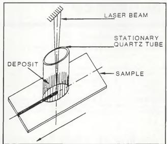
Fig. 1—Experimental setup for collection of vapors
