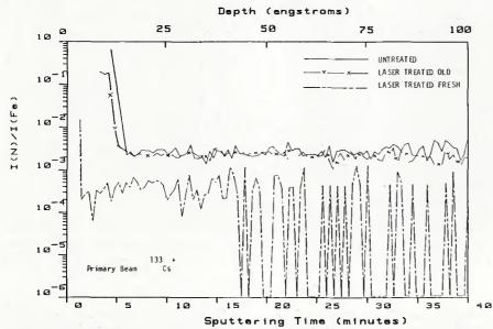
Fig. 8 – Relative counts of N/Fe as a function of sputtering time. Steel type: AlSl 202; primary beam: <sup>133</sup>Cs<sup>+</sup>; beam current: 1 nA; laser power: 600 W; welding speed:  $3 \times 10^{-3}$  m/s; helium flow rate:  $1 \times 10^{-4}$  m<sup>3</sup>/s
