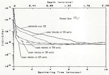
Fig. 7 – Relative counts of O/Fe as a function of sputtering time for samples welded at various laser powers. Steel type: AISI 202; primary beam:  $^{133}Cs^+$ ; beam current: 500 nA
