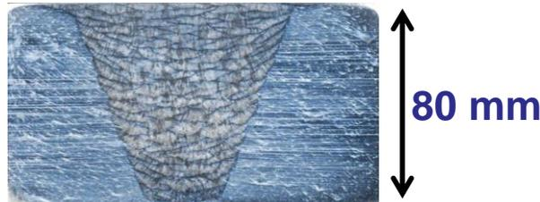
*Figure 2: Thick sections of Alloy 690 are joined with multi-pass arc welds. (Courtesy of EPRI)*
