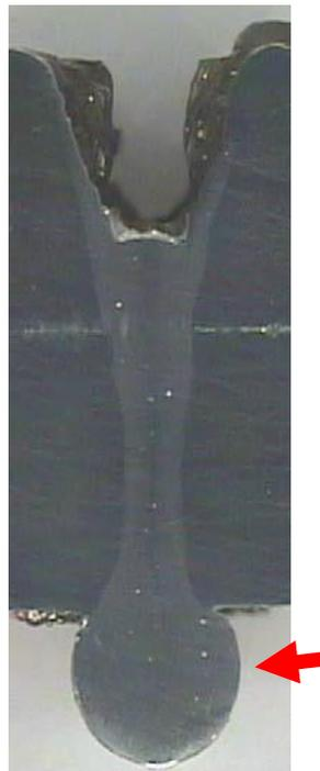
Figure 8: A root defect formed in a laser weld of 16 mm thick plate of 304 stainless steel [50].
