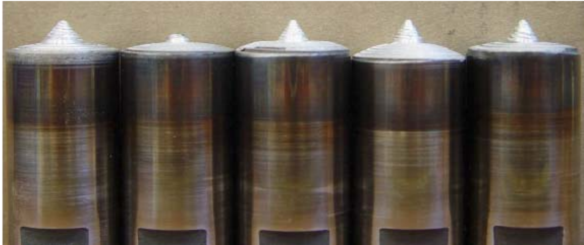
Figure 4.13 The tools used by Neilsen during FSW of AA7075 after the use. The tool pin in the second tool from the left sheared off during welding. [30]
